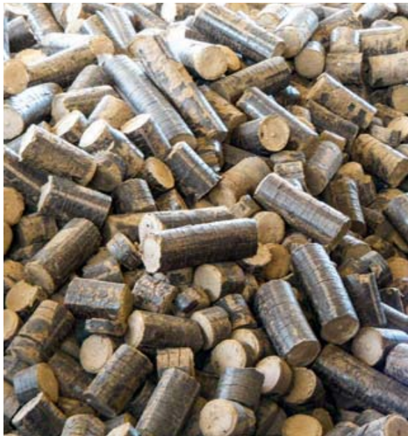
Biomass briquettes in India — solid biofuel pellets and briquettes can be produced from any biomass
