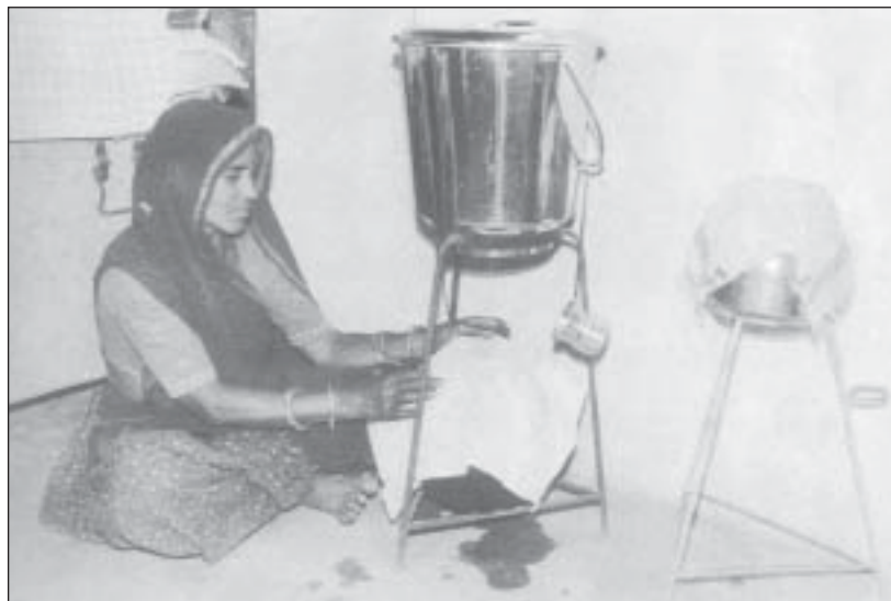
Photo 8.3: Fill-and-Draw Type Defluoridation Unit
