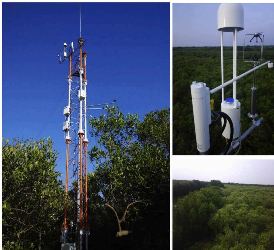
Fig. 2. Eddy covariance (EC) flux tower (left) in the dense area of Pichavaram mangrove forest. The CO 2 /H 2 O infrared gas analyzer system sensor and sonic anemometer and a part of the mangrove vegetation are shown in the right column upper and lower figures, respectively.
